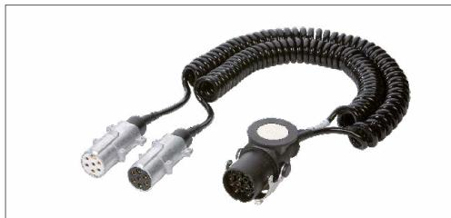
The 24 V adapters are used for the connection between towing vehicles (with 15-pin 24 V socket according to ISO 12098) and trailers (with 2x 7-pin 24 V sockets; 1x Type N or ISO 1185 and 1x Type S or ISO 3731). Especially helpful are these adapters for new trucks that are not factory equipped with 7P/24V sockets. The use of the adapter spirals ensures that an older trailer with 7P/24V system can be attached.
